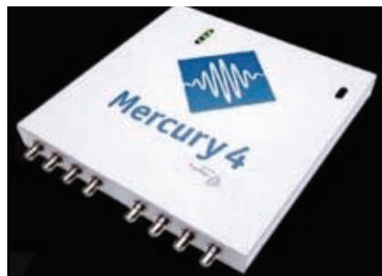
▲ Fig. 4 ThingMagic Mercury4 reader.
